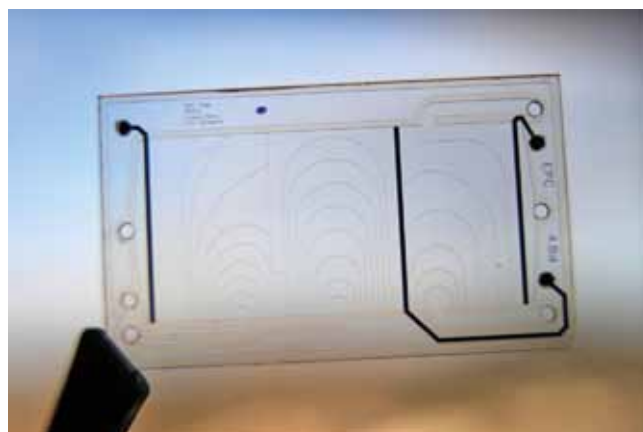
Abb. 3: Mikrochip des Lab-on-chip-Systems. Foto: Gregory Dame
